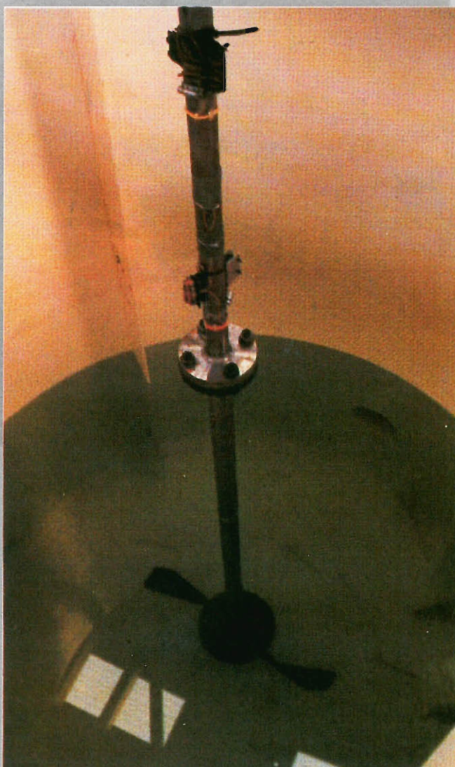
Laboratory strain gauge analysis on new impeller
